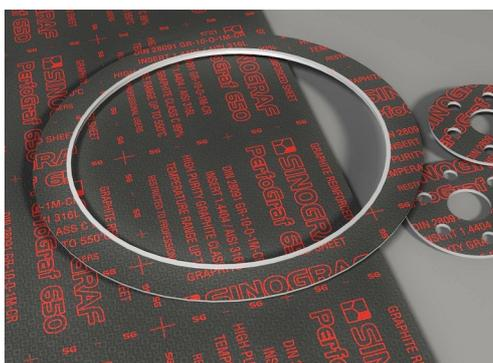
A following kind of sealing material is sheet made from pure, homogeneous graphite, which is rolled and strengthened by the planar orientation, sometimes by fibreglass insert, by carbon fibre possibly is reinforced by dispersed varies mineral fibres. This is material designed for lower parameters, in the low and middle range of
