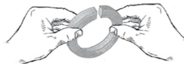
ring's proper settlement. Locks of each ring have to be each time moved by a certain angle, so as to distribute them evenly in the whole space and level formation of the package's weak points. To ensure gland's proper conduct, once the last ring is set, a place should remain, high at least at half the packing thickness.
