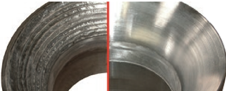
| Turning result of a special type valve seat
