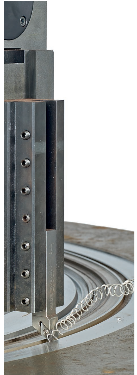
| Groove machining with the TDF-2 NC
